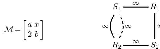
FIG. 4.1. Assume that a, b can take all values in [0, 1] and x can take all values in [-1, 1] . The SR graph associated with \mathcal{M} contains five edges. Positive edges are represented with bold lines, negative edges are represented with dashed lines. These conventions will be followed throughout.
