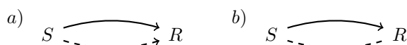
FIG. C.2. Two common double edge connections between vertices in a DSR graph. a) Increases in S may cause either an increase or a decrease in R , but S itself is unaffected by the interaction. b) Increases in S may cause either an increase or a decrease in R , and S is decreased by the interaction.
