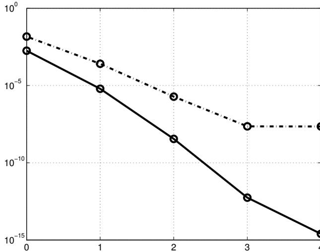
FIG. 8.7. The Goldstein-Taylor Model with the spatially varying  $\epsilon(x)$ : Error convergence in mean (solid lines) and standard deviation (dashed lines), with respect to gPC order for  $\epsilon_0 = 10^{-12}$ ,  $\Delta x = 0.01$ ,  $\Delta t = \frac{1}{12} \Delta x^2$ .
