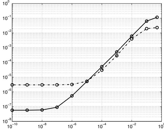
FIG. 8.10. *The Carleman Model: Errors in the mean (solid line) and standard deviation (dash line) of  $u$  by the gPC solution with order  $N = 4$  at varying  $\epsilon$  values. The reference solution is obtained by solving the limiting random diffusion equation (3.4).*
