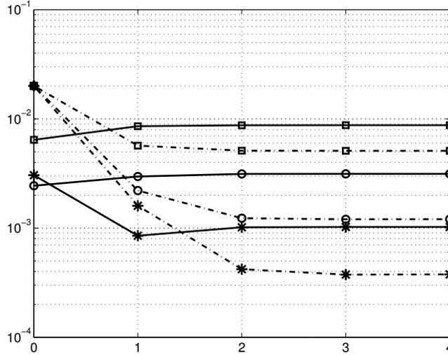
FIG. 8.13. *The linear transport equation: Errors of the mean (solid line) and standard deviation (dash line) of  $\bar{r}$  (circle) with respect to the gPC order at  $\epsilon = 10^{-8}$ :  $\Delta x = 0.04$  (squares),  $\Delta x = 0.02$  (circles),  $\Delta = 0.01$  (stars).*
