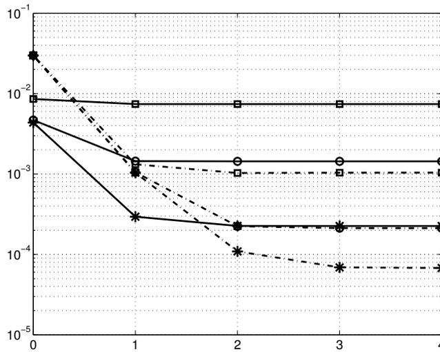
FIG. 8.3. *The Goldstein-Taylor Model: Error convergence in mean (solid lines) and standard deviation (dashed lines), with respect to gPC order for  $\epsilon = 10^{-12}$ . (Squares:  $\Delta x = 0.04$ , circles:  $\Delta x = 0.02$ , stars:  $\Delta x = 0.01$ ).*
