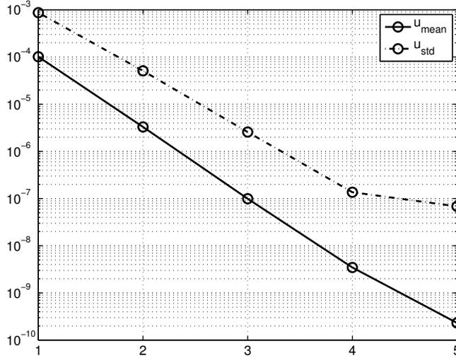
FIG. 8.17. The linear transport equation: Errors of the mean (solid line) and standard deviation (dash line) of  $\bar{\tau}$  with respect to gPC order, with the  $d = 5$  dimensional random input.
