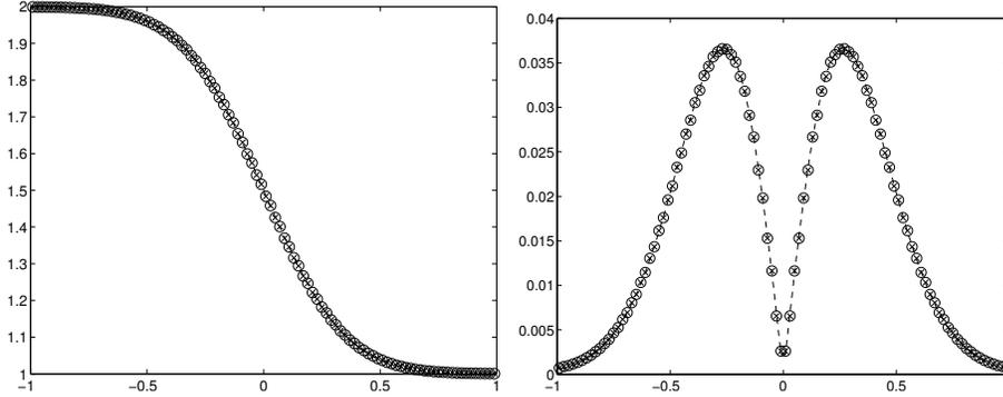
FIG. 8.2. *The Goldstein-Taylor Model: The mean (left) and standard deviation (right) of  $u$  with  $\epsilon = 10^{-12}$ , obtained by 4th-order gPC Galerkin (circles) and stochastic collocation (crosses), along with the analytical solution (8.2) (dashed lines) of the limiting diffusion equation (3.2).*
