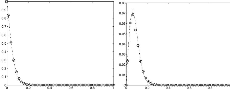
FIG. 8.14. *The linear transport equation: The mean (left) and standard deviation (right) of  $\bar{r}$  at  $\epsilon = 10^{-8}$ , obtained by the gPC Galerkin at order  $N = 4$  (circles), the stochastic collocation method (crosses), and the limiting analytical solution (8.6).*
