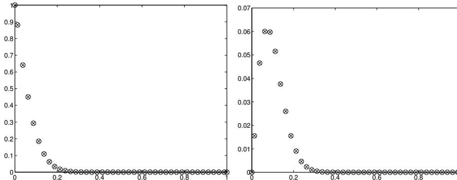
FIG. 8.16. *The linear transport equation: The mean (left) and standard deviation (right) of  $\bar{r}$  at  $\epsilon = 10^{-8}$ , obtained by 5th-order gPC Galerkin (circles) and the stochastic collocation method (crosses). The random input has dimension  $d = 5$ .*
