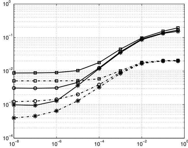
FIG. 8.15. *The linear transport equation: Differences in the mean (solid line) and standard deviation (dash line) of  $\bar{r}$  with respect to  $\epsilon^2$ , between the limiting analytical solution (8.6) and the 4th-order gPC solution with  $\Delta x = 0.04$  (squares),  $\Delta x = 0.02$  (circles) and  $\Delta x = 0.01$  (stars).*
