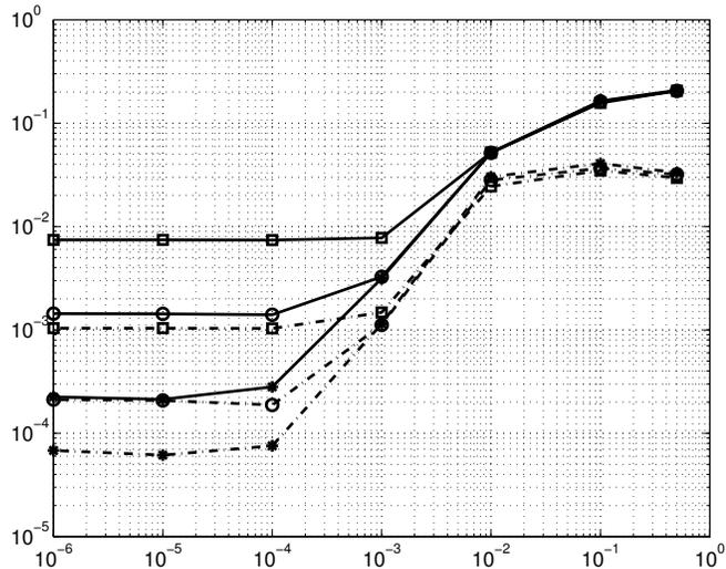
FIG. 8.4. *The Goldstein-Taylor Model: Differences in mean (solid lines) and standard deviation (dashed lines) with respect to  $\epsilon$  between the analytical solution (8.2) of the limiting diffusion equation (3.2) and the 4th-order gPC solution with  $\Delta x = 0.04$  (squares),  $\Delta x = 0.02$  (circles), and  $\Delta x = 0.01$  (stars).*
