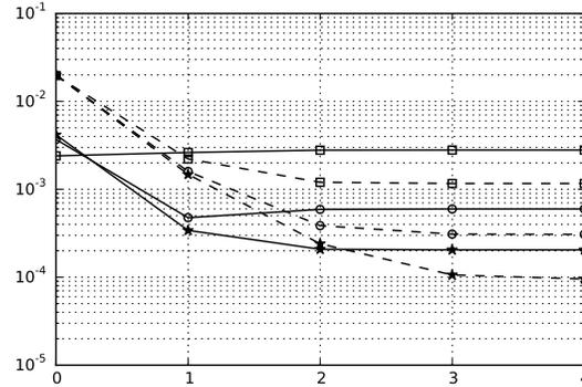
**Fig. 3** Example 3. Errors of the mean (solid line) and standard deviation (dash line) of  $\rho$  with respect to the gPC order  $M$  at  $\varepsilon = 10^{-8}$ :  $\Delta x = 0.04$  (squares),  $\Delta x = 0.02$  (circles),  $\Delta x = 0.01$  (stars).  $\Delta t = 0.0002/3$ .
