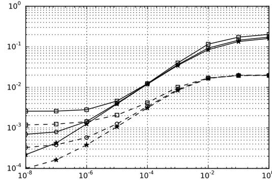
**Fig. 4** Example 3. Differences in the mean (solid line) and standard deviation (dash line) of  $\rho$  with respect to  $\varepsilon^2$ , between the limiting analytical solution (88) and the 4th-order gPC solution with  $\Delta x = 0.04$  (squares),  $\Delta x = 0.02$  (circles) and  $\Delta x = 0.01$  (stars).
