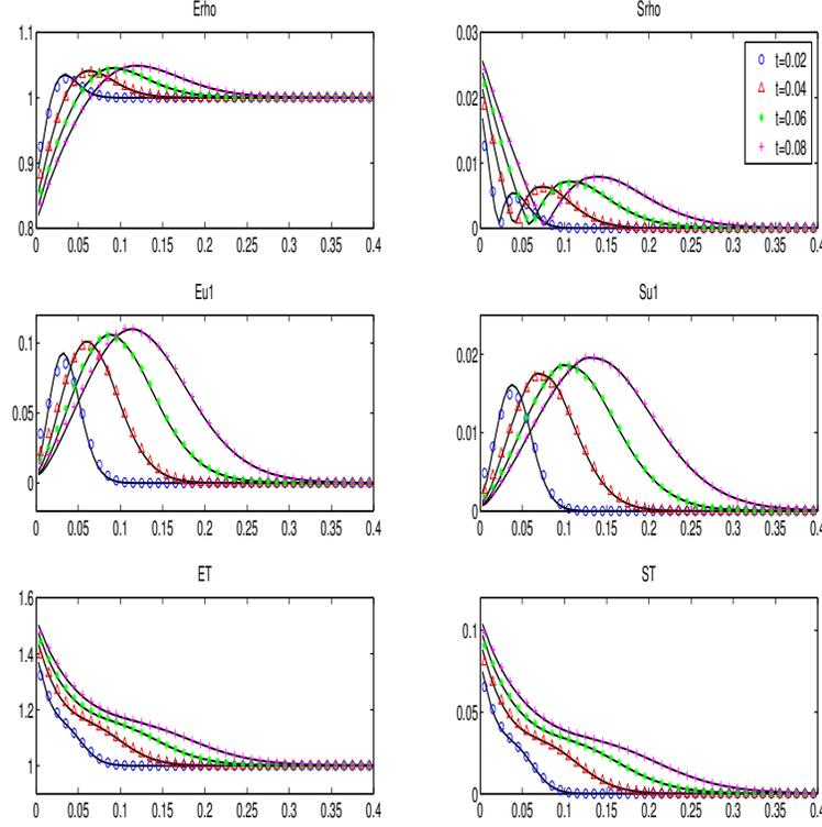
**Fig. 1** Example 1. Left column: mean of density, bulk velocity (first component), and temperature. Right column: standard deviation of density, bulk velocity (first component), and temperature. Solid line: stochastic collocation with  $N_z = 20$ ,  $N_v = 64$ ,  $N_\eta = 8$ ,  $N_x = 200$ . Other legends are the 7-th order gPC-sG solutions at different time with  $N_v = 32$ ,  $N_\eta = 4$ ,  $N_x = 100$ .
