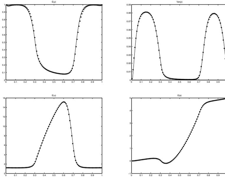
**Fig. 2** Example 2. First row: mean and variance of  $\rho$ . Second row: mean of velocity  $u$  and potential  $\phi$ . Time  $t = 0.05$ ,  $\Delta x = 0.01$ ,  $\Delta t = 10^{-5}$ ,  $\varepsilon = 0.001$ . Star: 4-th order gPC-sG solutions. Solid line: the reference solutions obtained by stochastic collocation.
